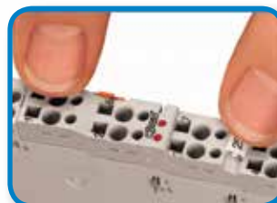
Place the connector into the I/O module
