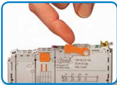
Locate the orange pull-tab on the connector...
