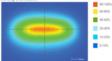
Optical measurement taken using AL-S025300M-WHI @ 300 mm
