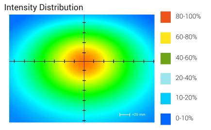
Optical measurement taken using AL116-WHIIC Rev. A @ 200 mm
